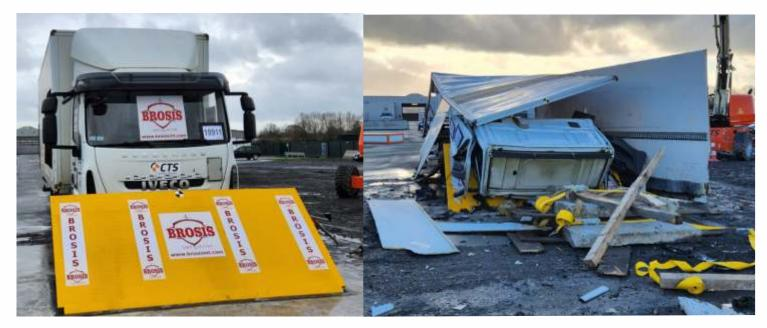
Brosis Sheild B12 is hydraulically operated Road Blocker that has been physically crash tested & certified according to IWA 2014-1:2013 from CTS, Germany. It is able to stop vehicle travelling at speed of 80km/hr carrying weight upto 7200 Kgs .It has achieved **ZERO PENETRATION** & fully **operational** post test.
