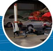
**PULL** with Shop-Hopper's 5-ton tower. SECTION with Chief's Universal Parts Holding. MEASURE during repairs for pinpoint accuracy.
